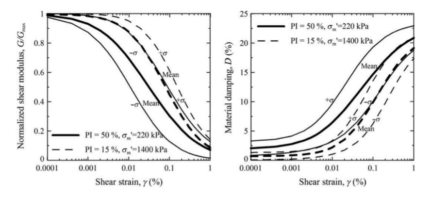
Example for Tertiary sediments 220 kPa /depth≈24m 1,400 kPa /depth≈130m
